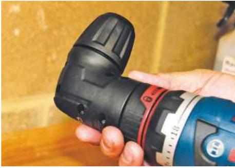
▲ Like the offset chuck it can be repositioned for better access
